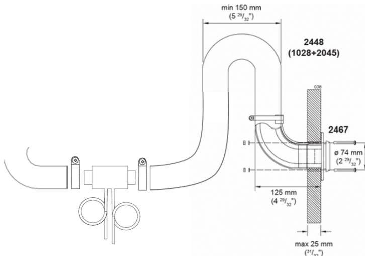
If necessary, a drainage lock can be installed into the exhaust pipe of a hull lead-through, but note the drainage lock must be positioned after the gooseneck.
