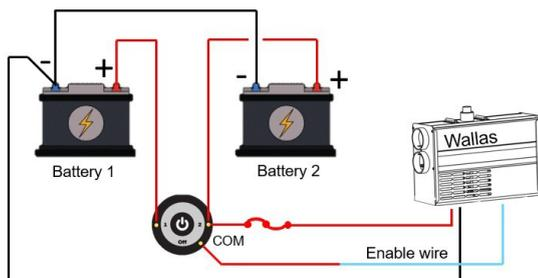
The blue wire should connect to the red +12V lead coming from the controlled side of the boat's main battery switch.
