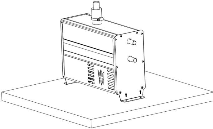
The heater can be installed to the floor by using "legs". Secure the device to a flat stable surface which is not tilted more than 5 degrees from the horizontal plane. While the device might not break if it is temporarily tilted to a steep angle (even for some hours) the burner will not yield optimal performance if it is constantly inclined. The "legs" and necessary screws can be found from the accessory bag.
