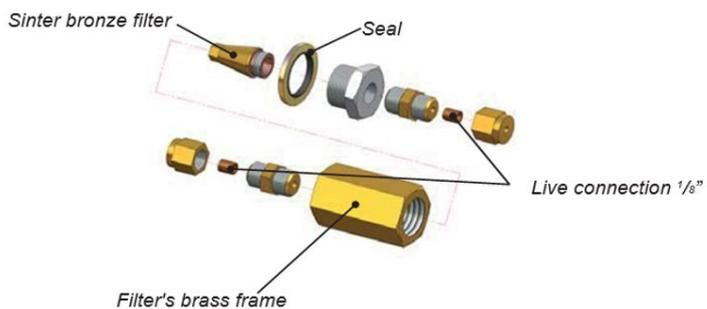
This filter is used in countries where a metallic fuel transfer system is required. A 1/8" metal pipe is used for the installation.
