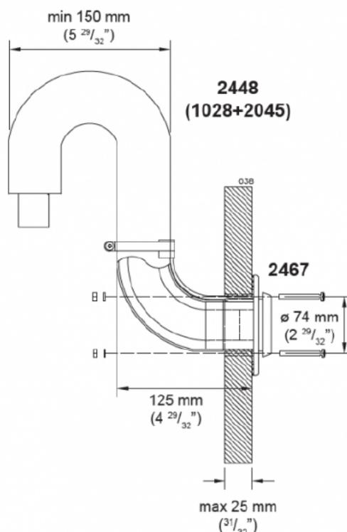
The **1028** exhaust gas pipe must be 30-50 mm (1 3/16" - 1 31/32") longer than the **2045** inlet pipe. This way the exhaust gas pipe will stay in place in the lead-through more firmly. The measurement depends on the overall length of the piping.
