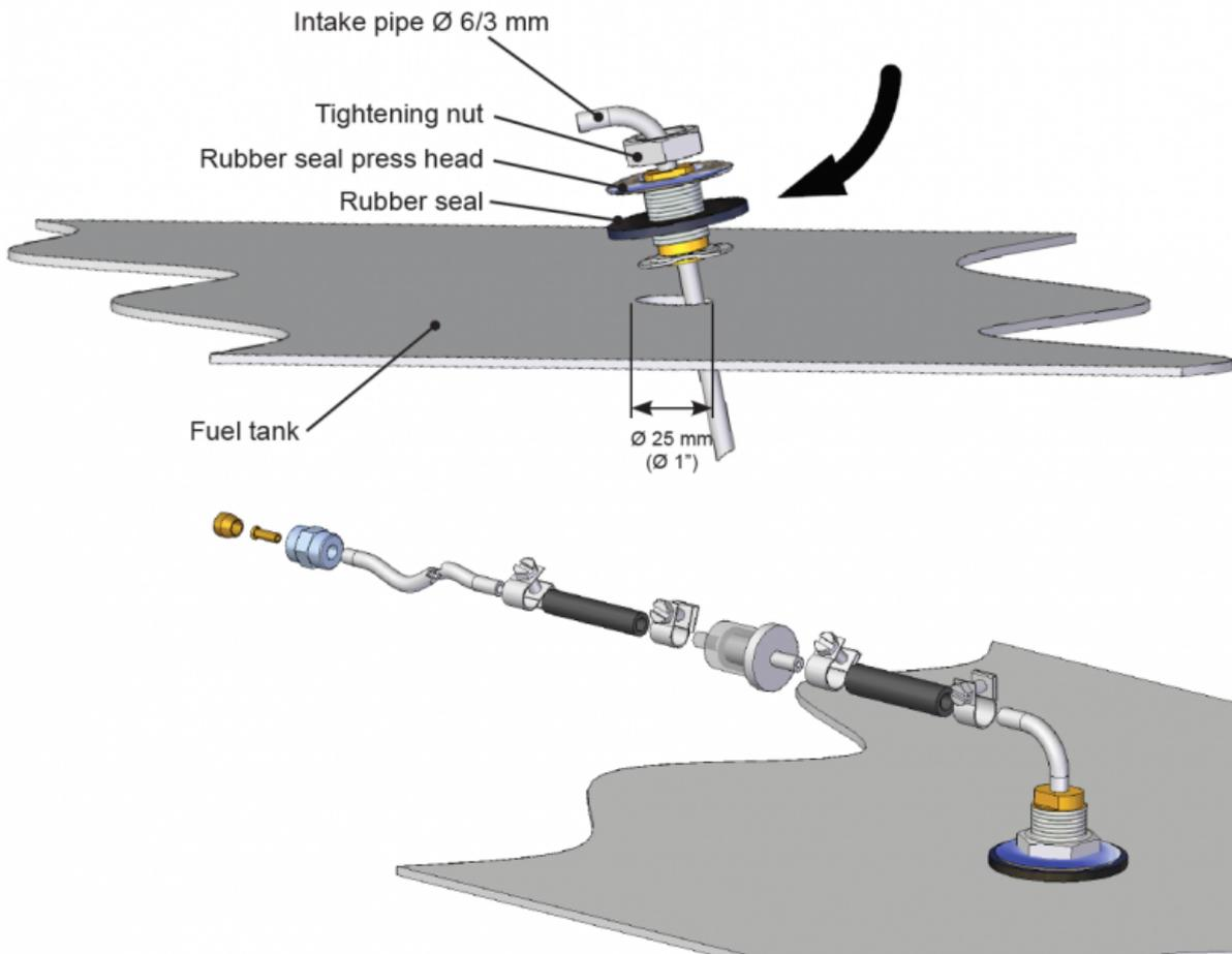
1. You will need to make a  $\varnothing 25$  mm (1") hole in the upper surface of the fuel tank. Choose the location of the hole so that when the fuel tank tilts the end of the intake pipe will stay in the fuel even if the tank is not full. If the end of the intake pipe does not reach the fuel, the device will quickly choke on the air in the fuel system and that can cause malfunction to the system.
