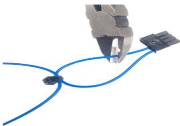
Locate the blue Enable wire loop what is connected to bottom of the heater.
